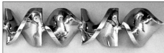
Each element is a rectangular plate twisted 180°. Right and left elements are joined alternately at 90° angles to each other.
