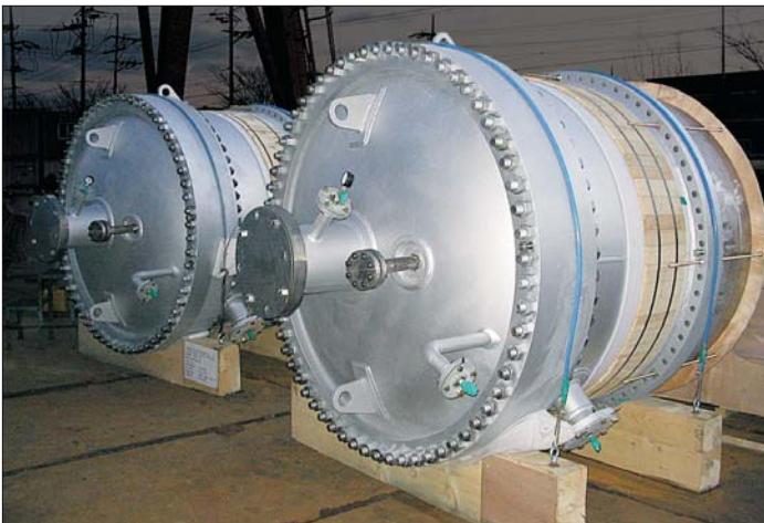
Devolatilization preheaters, each containing 1,890 tubes and providing 3,638 ft 2 (338 m 2 ) surface area
