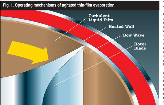
spirals down the wall while bow waves developed by the rotor blades generate highly turbulent flow and optimum heat flux (Fig. 1). Volatile components evaporate rapidly. Vapors can flow either cocurrently or, more commonly, countercurrently, and are ready for condensing or subsequent processing as they leave the unit.
