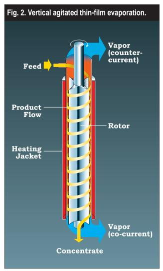
Agitated thin-film evaporation systems are widely used in the distillation of high-boiling and temperature-sensitive organics.
